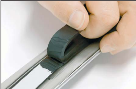
Picture 10: Peel adhesion test
