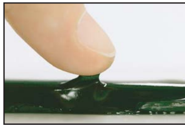
Pictures 7 - 9: Press the finger tip lightly on the adhesive and lift off. The skin time is the point at which the adhesive no longer sticks to the finger (image on the right).
