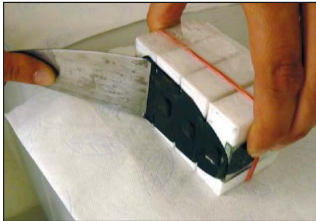
Picture 14: Removal of excess of silicone adhesive
