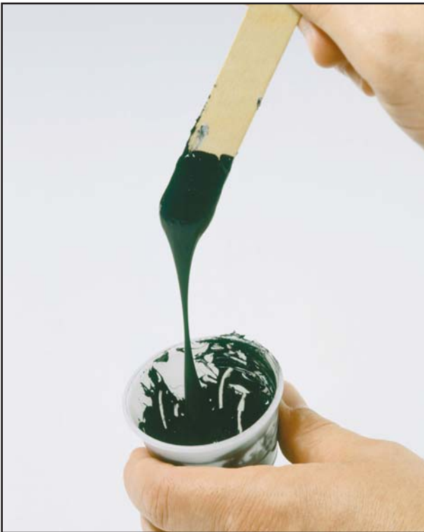
Picture 5: Material shows paste-like behaviour: snap time not yet reached
