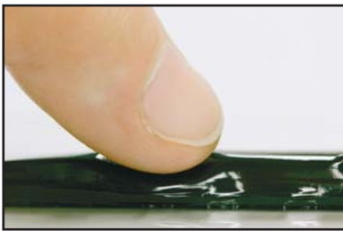
Pictures 7 - 9: Press the finger tip lightly on the adhesive and lift off. The skin time is the point at which the adhesive no longer sticks to the finger (image on the right).
