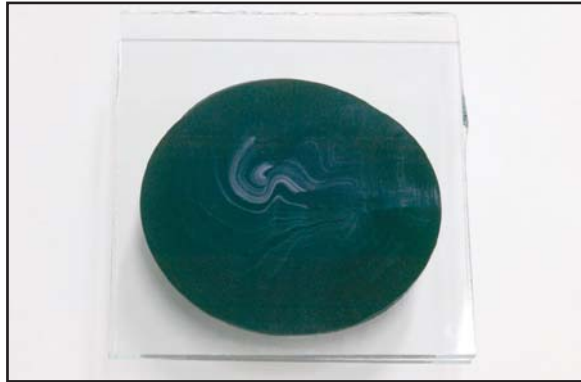
Picture 2: Negative test = inadequate mixing
