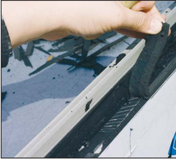
Picture 17: Good adhesion, deglazing test positive
