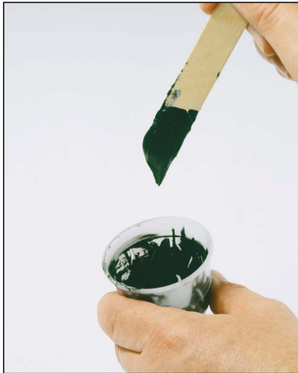
Picture 6: Material shows rubber-like behaviour: snap time reached
