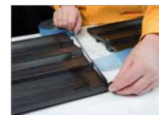
Applying the adhesion strip
