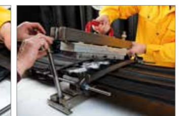
Powdering of waterstop and inserting into the vulcanizing equipment
