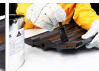
Applying the vulcanizing solution to the rubber surface
