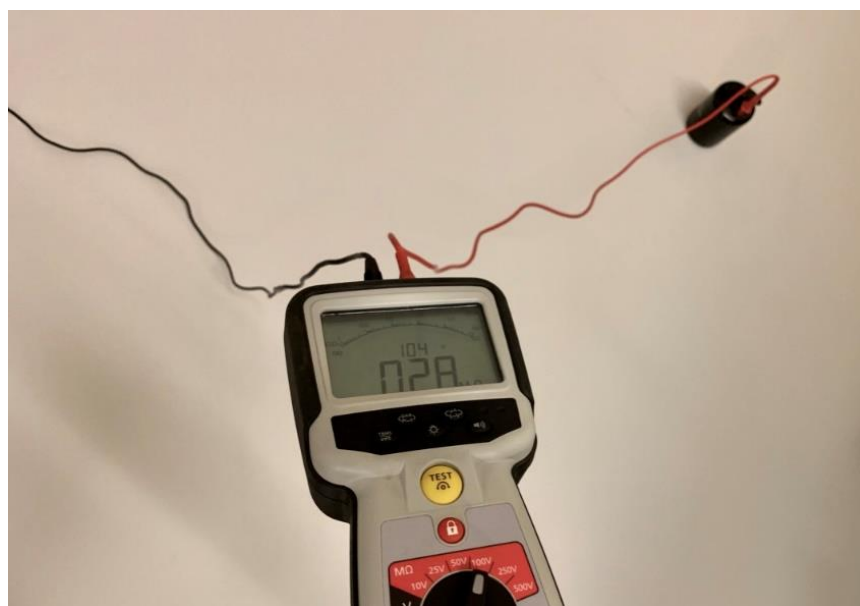
Figure 6: Resistance to ground measurement on the flooring under test
