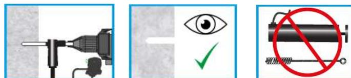
1. Use the specified hollow drill bit and follow the manufacturers instruction. Ensure the vacuum system is on.
