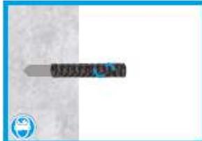
Insert the rebar, free from oil or other release agents, to the bottom of the hole using a back and forth twisting motion ensuring all the threads are thoroughly coated. Adjust to the correct position within the stated working time.
