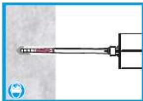
Insert the mixer nozzle (resin stopper / extension tube if applicable) to the bottom of the hole. Begin to extrude the resin and slowly withdraw the mixer nozzle from the hole ensuring that there are no air voids as the mixer nozzle is withdrawn. Fill the hole to approximately  $\frac{1}{2}$  to  $\frac{3}{4}$  full and remove the mixer nozzle completely.
