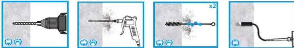
1. After drilling the hole, Blow 2 times from the back of the hole with oil-free compressed air (min. 6 bar) until return air stream is free of noticed dust. Repeat this action twice.
